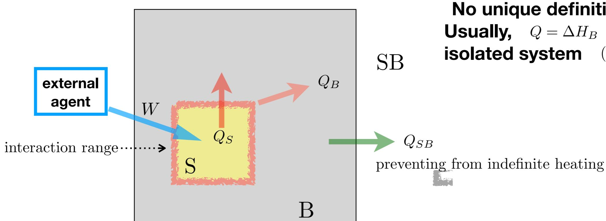
First laws  $\Delta H_S = W - Q_S$     $\Delta H_B = Q_B - Q_{SB}$     $\Delta H_{tot} = \Delta H_S + \Delta H_B + \Delta H_I = W - Q_{SB}$
