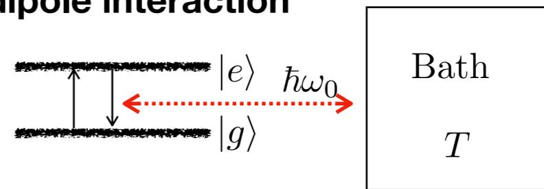
$$\sigma_1 = |e\rangle\langle g| + |g\rangle\langle e|, \quad \sigma_2 = -i(|e\rangle\langle g| - |g\rangle\langle e|), \quad \sigma_3 = |e\rangle\langle e| - |g\rangle\langle g|$$
