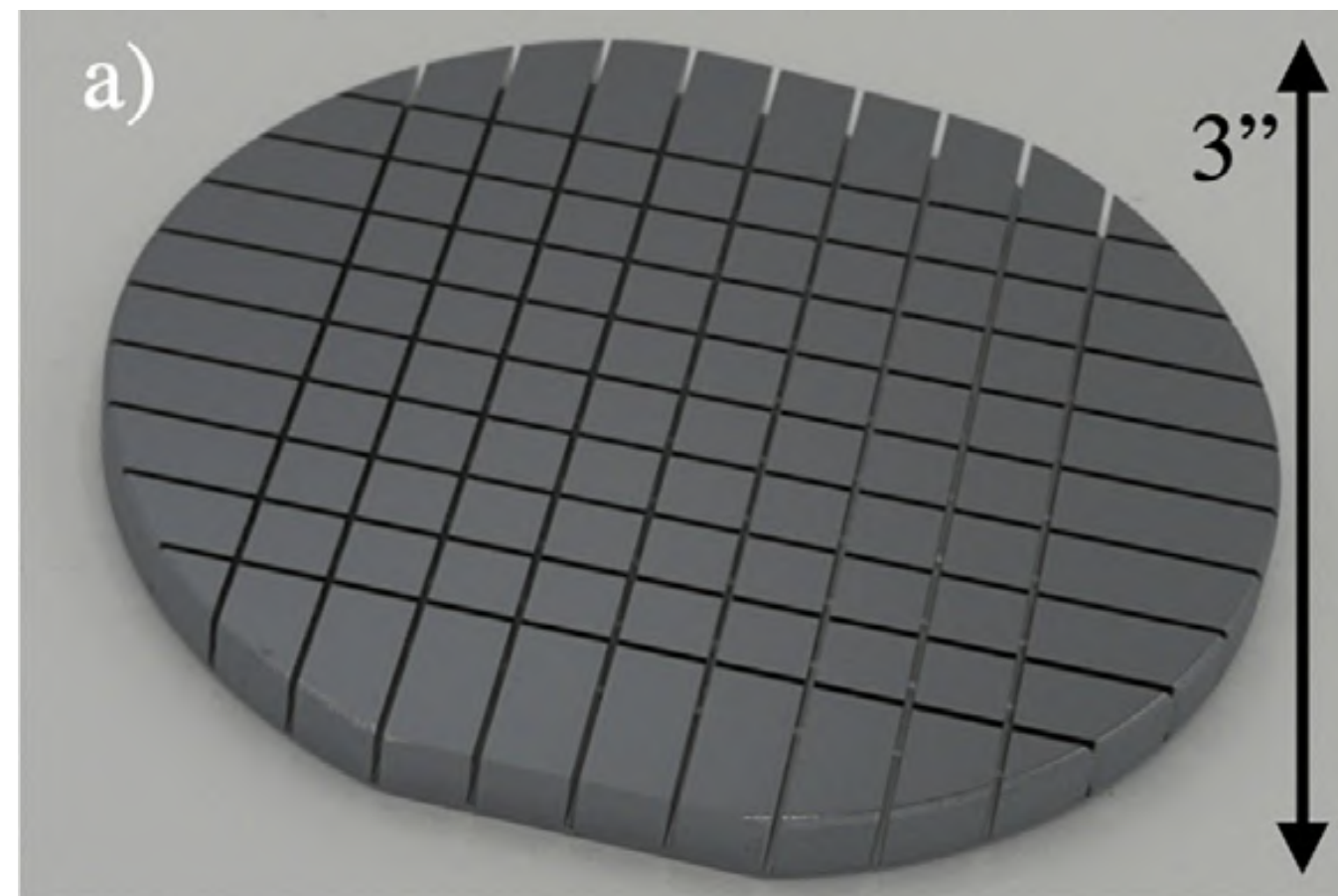
Demonstrator: 60 detectors (KIDs) for 3" wafer
