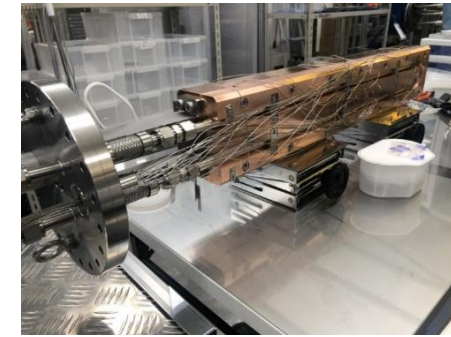
Cooling test of shielding (Cu for Phase-I)
