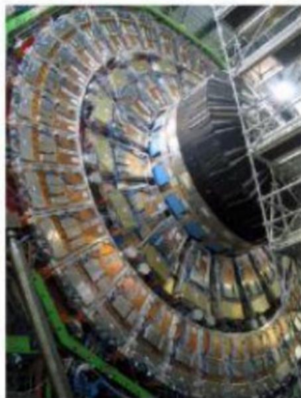
The ME1/3 CSC's new cover the RPC outer ring and hence complete the first Muon station on YE+1.
