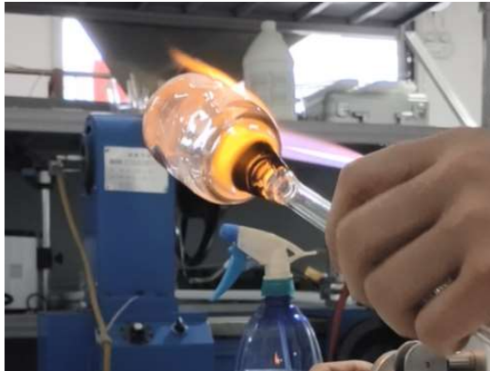
1. In-house ^3\text{He} cell fabrication and filling
