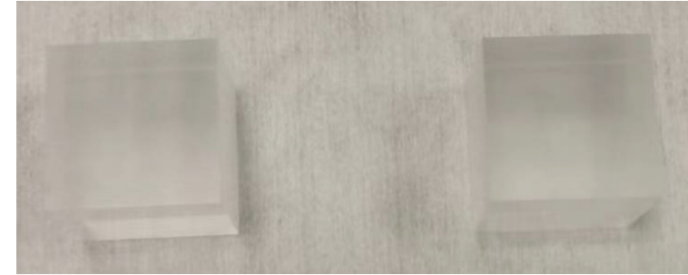
Transmittance (without correction of reflection) : \sim 84\% @420 nm
