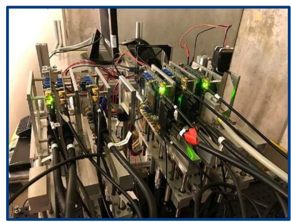
Characterization of potential electrode material with e<sup>+</sup> and  $\mu^+$
