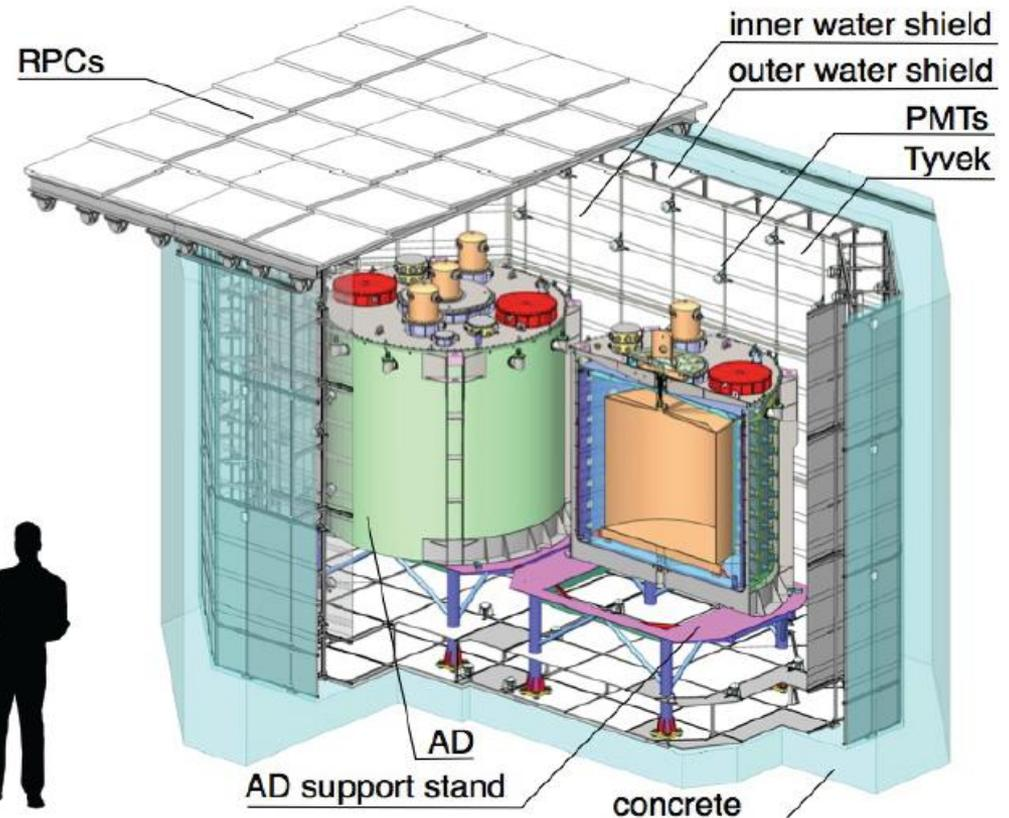
Two-zone ultrapure water Cherenkov detector
