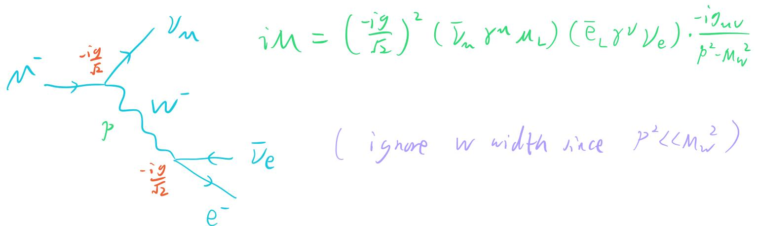
For  $p^2 \ll M_W^2$ , we can expand the operator
