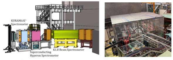
(*K*<sup>−</sup>, *K*<sup>+</sup>) reaction events are tagged by the K1.8 beam and the KURAMA spectrometers.
