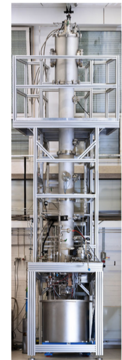
Krypton distillation column
