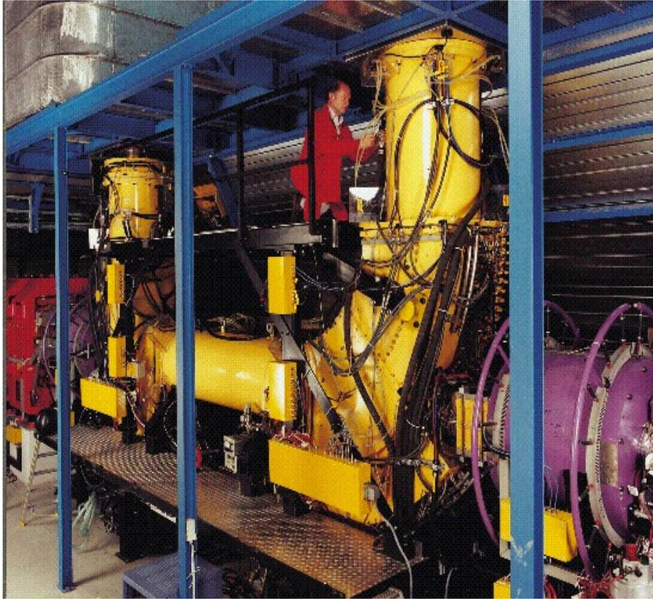
momentum exchange with 'cold', collinear e- beam. The ions get the sharp velocity of the electrons, small size and divergence
