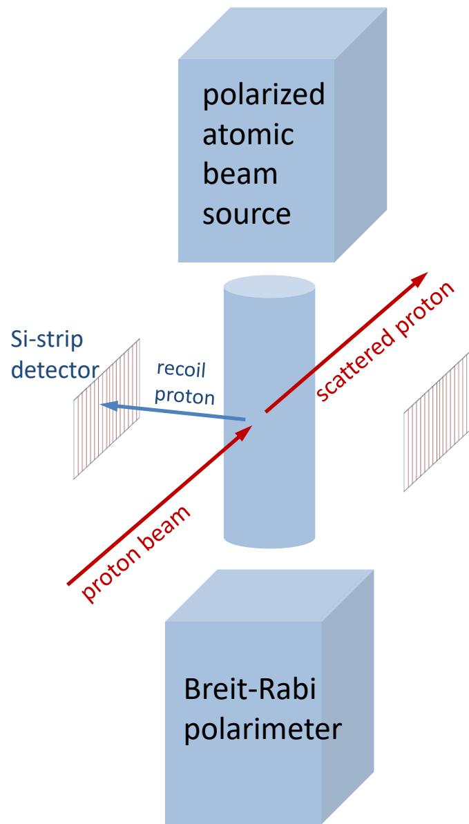
The H-Jet polarimeter at RHIC
