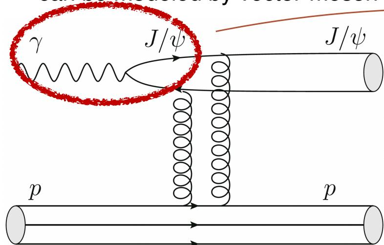
$$\frac{d\sigma_{\gamma N \rightarrow J/\psi N}}{dt}(s, t=0) = \frac{3\Gamma(J/\psi \rightarrow e^+e^-)}{\alpha m_\psi} \left( \frac{k_{J/\psi N}}{k_{\gamma N}} \right)^2 \times \frac{d\sigma_{J/\psi N \rightarrow J/\psi N}}{dt}(s, t=0)$$
