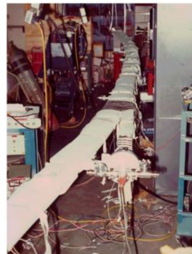
Figure 24. SPEAR bending magnet vacuum chamber with the 1st port to extract synchrotron radiation for experiments (Herman Winick collection).
