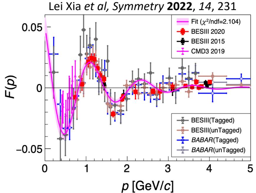
$|G_{\text{eff}}|$  data are fitted with the model: the **monopole decrease** with a **damped oscillation** : *E. Tomasi-Gustafsson et al., PRL. 114, 232301 (2015), PRC 103, 035203 (2021)*
