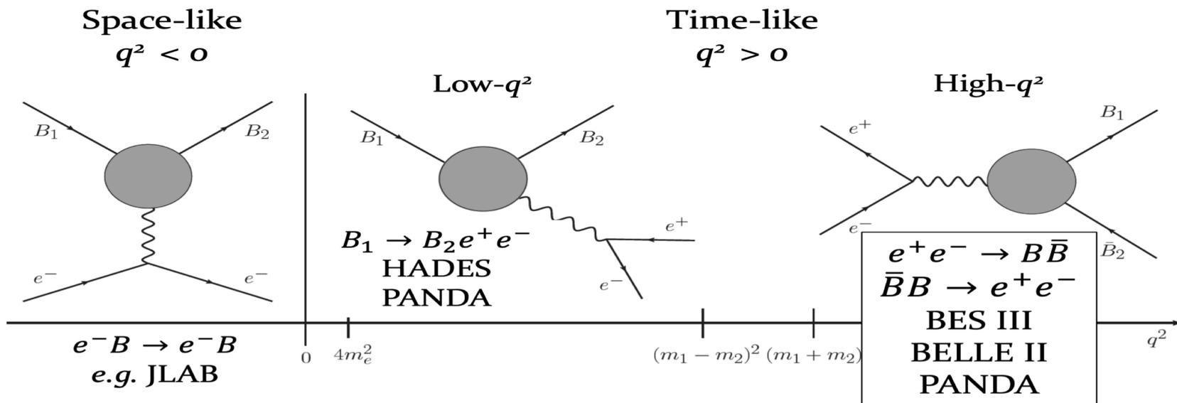
The nucleon **electromagnetic vertex**  $\Gamma_\mu$  describing the hadron current:
