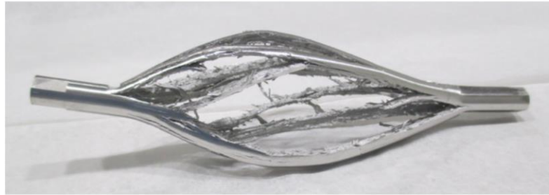
Ir rod after a single proton pulse ( 1.27 \times 10^{12} pot) Torregrosa et al. 2016. CERN-EN-2016-004
