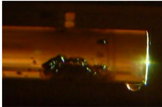
NuMI-MINOS target cooling water leak and radiation-assisted corrosion, FNAL
