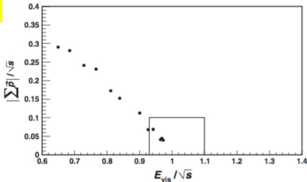
FIG. 3. A scatter plot of  $E_{\text{vis}}/\sqrt{s}$  versus  $|\sum \vec{p}|/\sqrt{s}$  for the  $J/\psi$  lata. The indicated signal region is defined as  $0.93 \leq E_{\text{vis}}/\sqrt{s} \leq 1.10$  and  $|\sum \vec{p}|/\sqrt{s} \leq 0.1$ .
