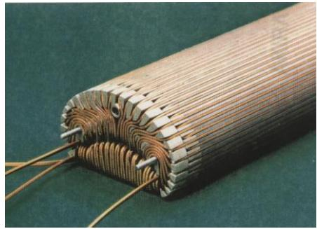
Truncated double cosine theta superconducting septum magnet
