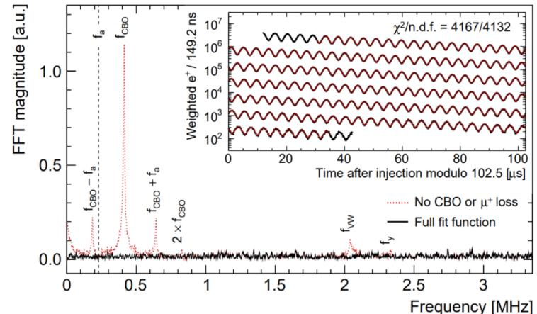
$$N_x(t) = 1 + e^{-t/\tau_{\text{CBO}}} A_{N,x,1} \cos(\omega_{\text{CBOT}} t + \phi_{N,x,1}) + e^{-2t/\tau_{\text{CBO}}} A_{N,x,2} \cos(2\omega_{\text{CBOT}} t + \phi_{N,x,2})$$
