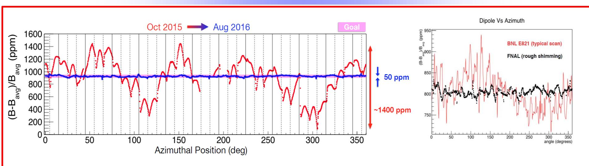
Shim 1.45 T field to high uniformity and measure it vs time
