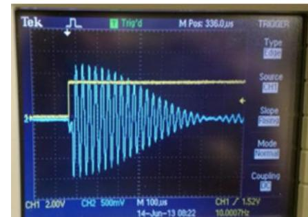
(FID) Waveforms with ~10 ppb resolution
