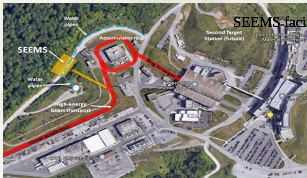
Figure 2. Overhead schematic showing the potential layout of the combined \mu SR/SEE facility. Some shielding and beamline-----components have been omitted for clarity.
